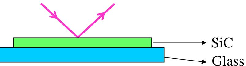
In the EUV the best R is obtained with CVD SiC coatings, that are prepared at high substrate temperature.
