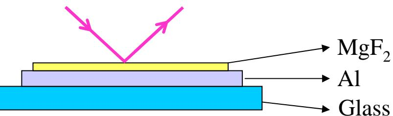
Al is the material with highest R down to 83 nm. After air exposure it becomes useless in the VUV.
