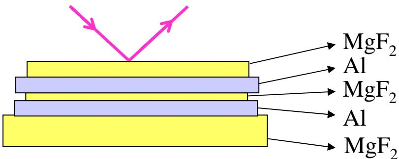
The variation of layers thickness allows tuning and out-of-band rejection.
