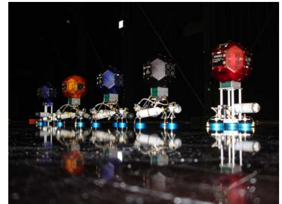
Five SPHERES on air carriages on MSFC Flat Floor
